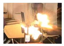
FIGURE 1. Lithium ion battery explosion on aircraft.
