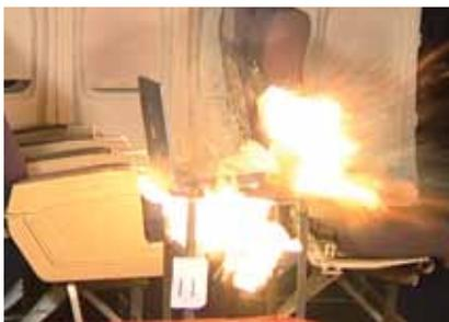
**FIGURE 1.** Lithium ion battery explosion on aircraft.
